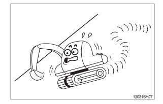
The engine angularity limits are 30 degree. Do not operate by more than the engine limits in any case.
