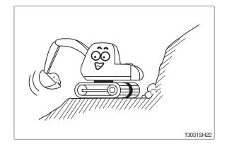
The swing on the slope can be danger of rolling over.
